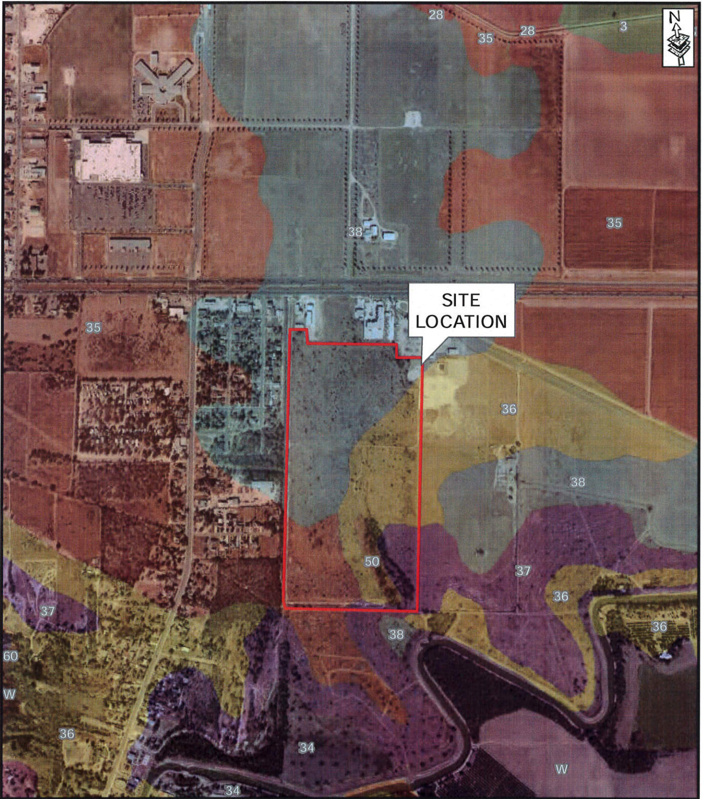
Figure 3 L&G Consulting Engineers La Joya Watershed Phase I - Task B Soil Classification Map USDA SOIL CONSERVATION SERVICE
